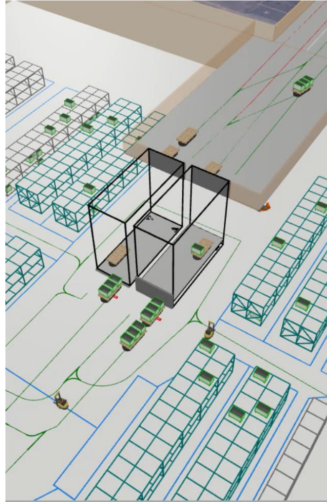
Two bidirectional single lifts
