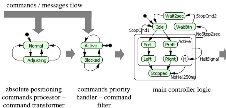
Figure 3 Command pipelining
