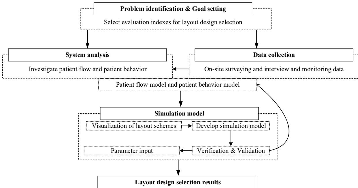
Figure 1: The process of layout design selection.
