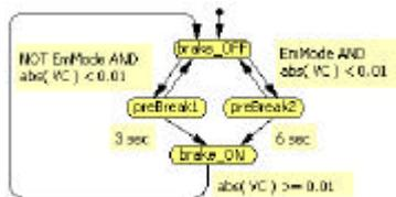
Brake control was implemented in the control block using statechart notation (see figure left). If the condition for activating the brake is true it switches to the `preBrake` state.
