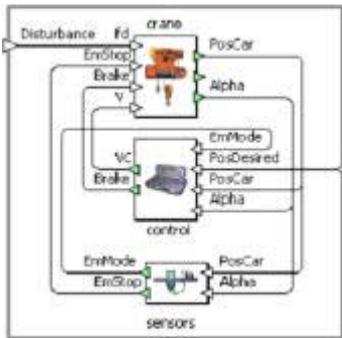
The crane object consists of the crane-mechanics and the DC-motor. The mechanics of linear and nonlinear systems, as well as the DC-motor were implemented plainly using given equations. The control block generates voltage for the motor and switches on/off brakes, whereby discretisation is implemented by triggering the block with the sampling time. This object receives information about car status and car desired position. The sensors object implements checking and control of any emergency modes.
