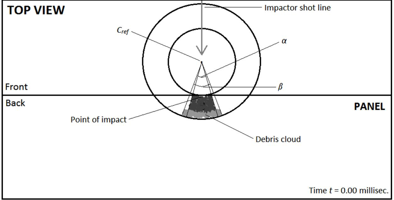
**Figure 4** Screenshot of BISM’s 2D “top view” animation window at simulated time zero, showing the debris fragments lying within a section of the outlined spherical shell. The panel fragments (light gray) lie in front of the residual impactor and its spall fragments (dark gray).
