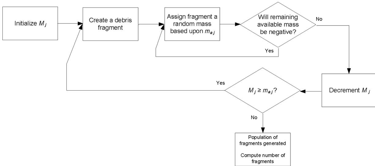
**Figure 3** Flowchart of the logic for impactor spall and panel fragment generation in BISM.
