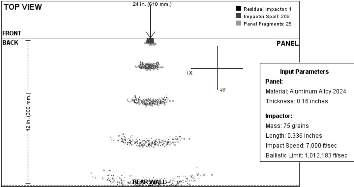
Figure 5 A screenshot of the 2D “top view” animation window during a simulation run.
