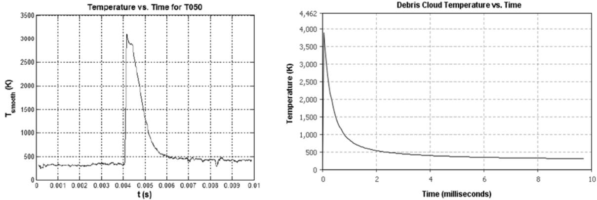
**Figure 8** (Left) temperature time series for test shot T050 from Buck *et al* (2011), time of impact = 4 milliseconds; (right) temperature time series obtained from a BISM run, time of impact = 0 milliseconds.
