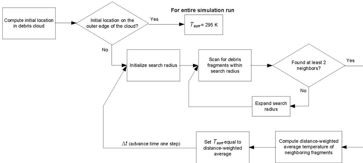
**Figure 7** Flowchart logic for updating the surrounding temperature,  $T_{surr}$ , of each fragment.
